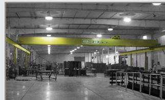
We have a multi-hook overhead crane system with a 25-ton lift capacity that spans 72' x 320' of our manufacturing floor space with easy transport access, allowing us to handle large projects. We also have a 10-ton vacuum lift, which allows us to handle the metal without causing scratches.
